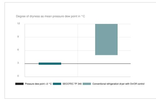
refrigeration dryers, on the other hand, ensure material-friendly operation thanks to their high thermal storage capacity. Once the thermal mass has been charged, the refrigerant compressor and fan motor can remain switched off for much longer without impacting pressure dew point stability.
